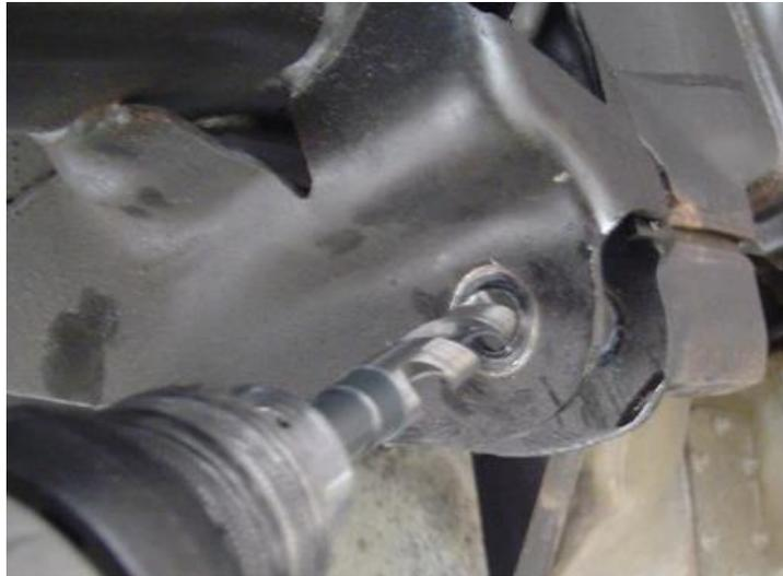
**Drill Out the OEM Track Bar Mount to 5/8 or Make Sure the Hole Passes a 5/8 Bolt**
