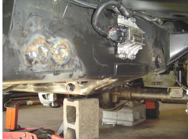
**Module Relocation and Crush Sleeves Welded**
