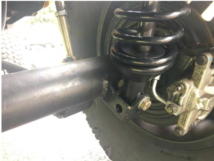
**Note:** The distance between these two mounts will need to be 52.375" (center of one mount to center of the other mount). The wider the better as long as there is no interference.
