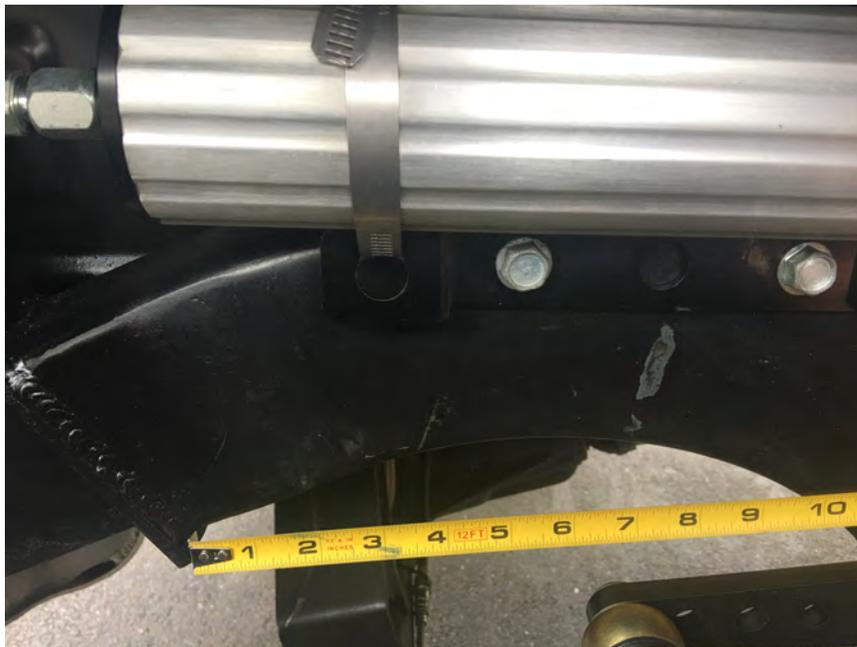
French in the mount deep enough so the edges stick out only 3/8 so you can get a nice 1/4" fillet weld all the way around the mount. The front leading edge of the mount should be
