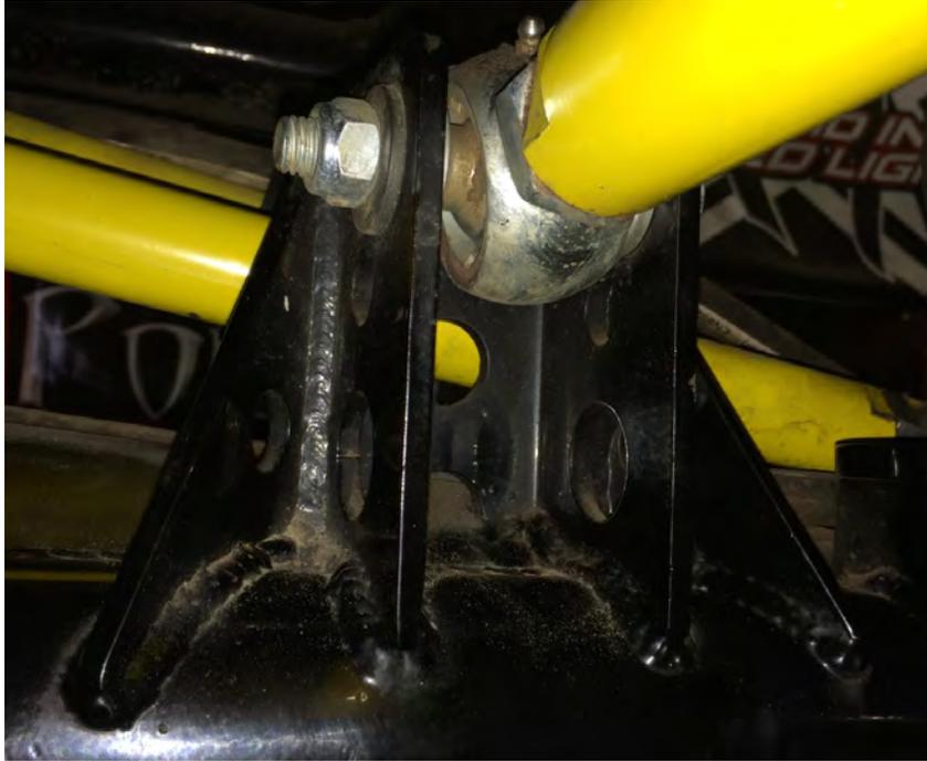
**Note:** To set the placement of the **Trail Runner Upper Control Arm Mount** either set the mount one of two ways. Position the new mount in the same position as the factory passenger side upper mount if you are swapping in JK axles. If your axle does not have this mount factory then set your caster to the axle manufactures specs and then set the front face of the supplied bracket vertical.
